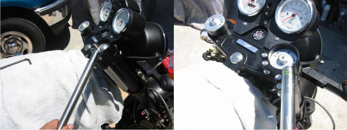
STEP 5. There is a 12mm gap between the top of the Convertibars Cyclops clamp and the top of the fork leg. If the fork legs are raised in the triple trees to provide the Cyclops clamp full purchase on the fork legs the handing will change on the bike. OR mount the Cyclops clamp under the top clamp.
