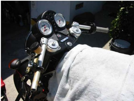
STEP 3. At this time cover the tank to protect it from scratches and remove the left grip and controls from the stock clip on bars.
