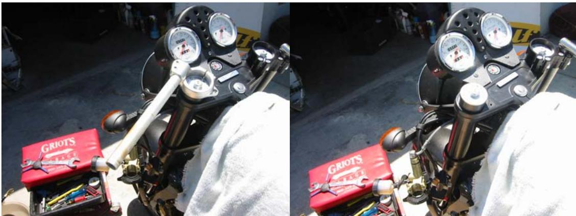
STEP 4. Remove the 5mm Allen screws securing the clip on bars to the top clamp. Loosen the 6mm screws on the clamp that secure the bars to the fork leg – remove the bars.
