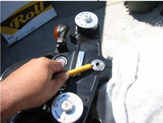
STEP 7. Remove the 3- 6mm pinch screws from the top clamp. Remove the plastic cover hiding the 8mm top nut and remove the top clamp. Install the Cyclops clamps under the top clamp.
