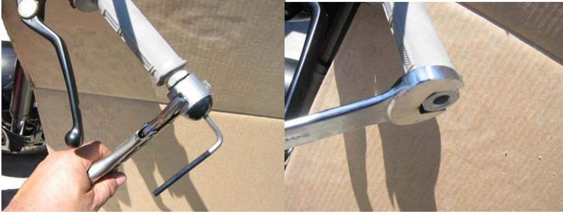
STEP 2. Using a 24mm wrench remove the end cap plug.
