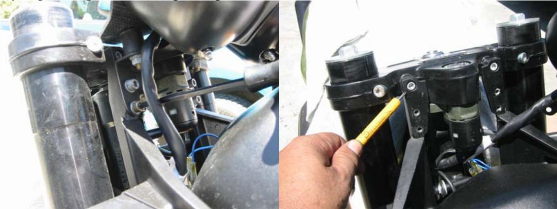
STEP 6. Remove the instrument cluster by removing the 4-5mm screws located below the Speedo. Remove the 4-5mm screws securing headlight mounts to the triple trees and move the control line to a position between the fork leg and the headlight mounts.
