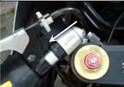
4. Rotate Lever/Handlebar, collet, and bolt plate together to a new indexed position
