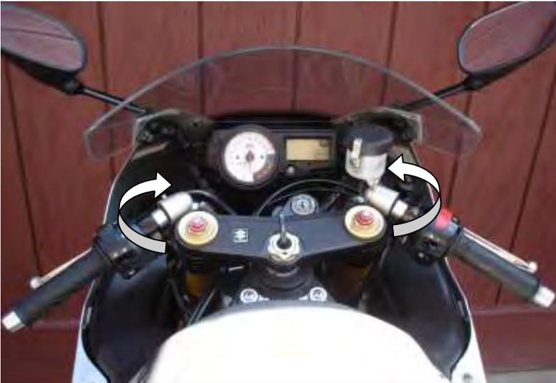
Tighten Cyclops clamp on the fork first,
