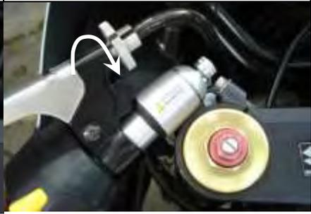
3. With a firm grasp, grip & flex the handlebar up and down until the collet pops out
