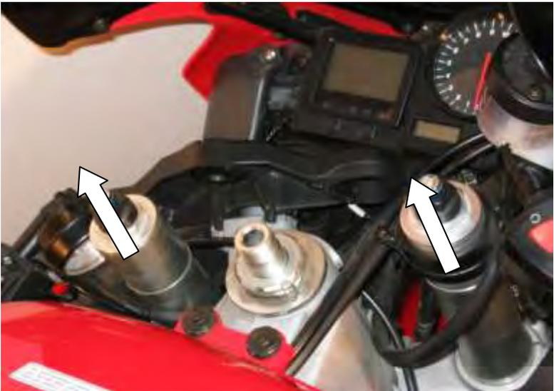
**Step 8.** Install the Cyclops clamps as in photo. Mounting the clamp flipped over is optional.
