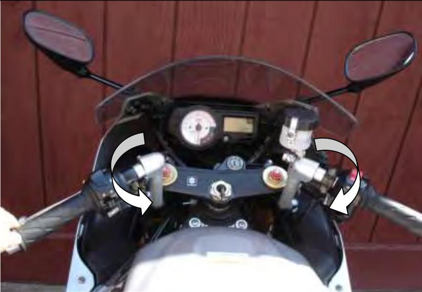
Tighten Cyclops clamp on the fork first,
