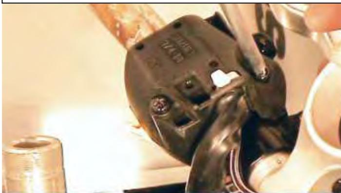
**Step 5.** If the installation requires installing under the triple clamp, loosen and or remove the two triple clamp pinch bolts and one main nut.
