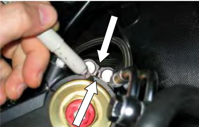
**We do NOT recommend altering the factory Steering stops. Only if absolutely needed, use fairing spacer pack or other lifting components to lift fairing for more handlebar rise.**
