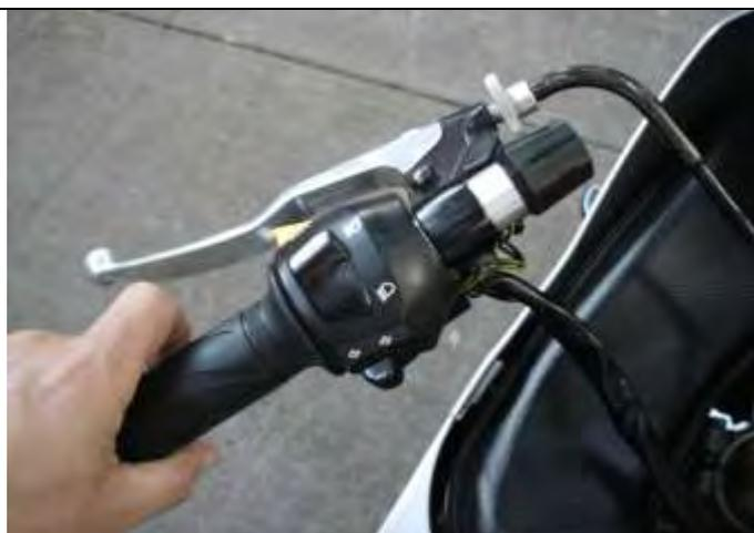
**Step 14.** Bolt the handlebar together using the washer or reservoir mount
