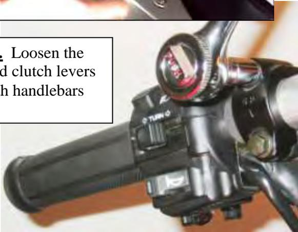
**Step 4.** Loosen 2 screws on each switch box.
